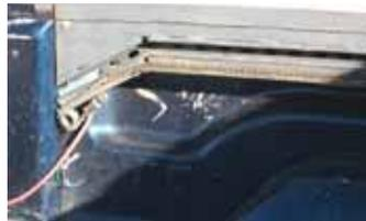
Track angles down at rear of box to tip tool box backwards.
