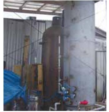
Dick Carrier's home-built, 400-gal. biodiesel processor uses waste cooking oil from restaurants as the base product.
