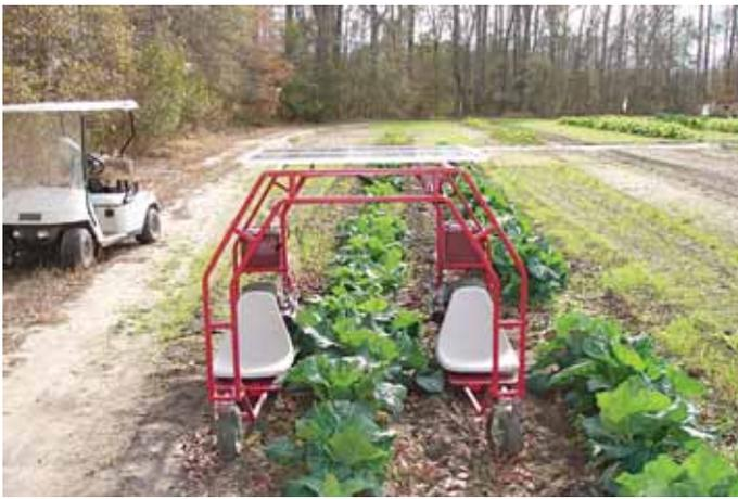
Randy Graham used parts from a powered wheelchair to build this sit-down, solar-powered picking machine.
