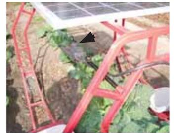
Joystick control (see arrow) is mounted just overhead and can be moved from one side of cart to the other.
