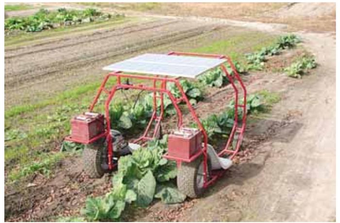
Unit works like a zero turn riding mower in that the front wheels swivel as the larger rear wheels control the turn.
