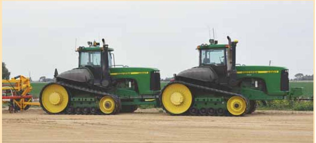
To increase planting capacity on their 47,000-acre operation, the Zells joined two Deere 9400T tractors to work as a single unit.
