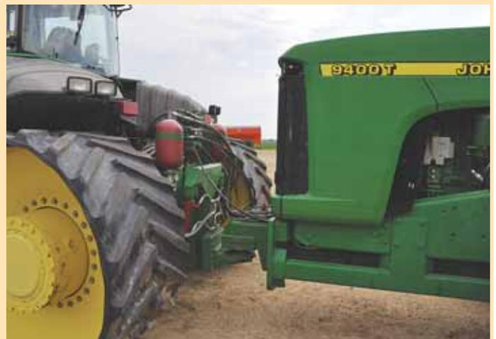
Hitch system between tractors uses a pair of hydraulic cylinders and accumulators to dampen up and down movement. A hitch frame runs back to the drawbar on the rear tractor. It's braced to the rear tractor frame with steel plates.
