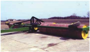
Tim Kelly used three 14 1/2-ft. long, 3-ft. dia. sections of steel oil pipeline to build this field roller.
