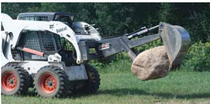
Moving big rocks is no problem for the heavy-built GrappleHoe that quick-taches to your skid loader or front-end loader.
