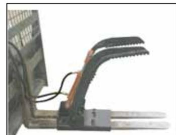
Fork Grapple is designed to slip onto a set of loader forks set close together.
