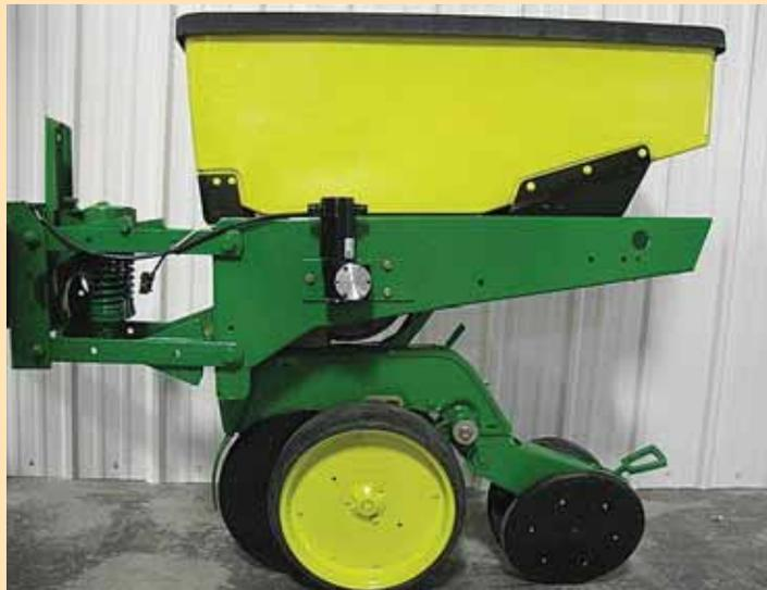
Electric motors are used to drive planter's seed plates. Each motor is controlled by a microprocessor-based drive system, which results in more precise seed placement.
