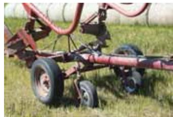
Front hitch is attached to square beam frame with 4 bolts (left). A 10-ft. long drill pipe runs from push plate on beam back to quick-tach frame on loader.
