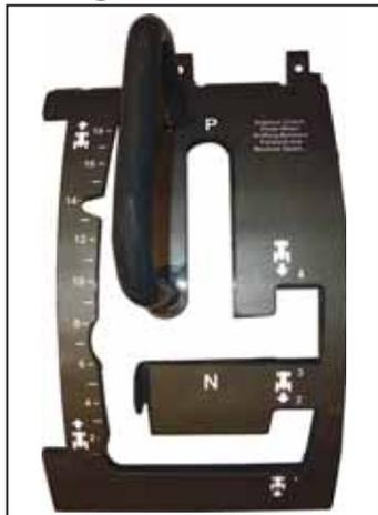
Shift kit includes a lock lever that blocks off the lower 6 gears to shorten up your shift movements.
