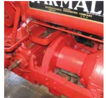
He kept the starting system hidden as much as possible. Starter motor mounts inside tractor's frame rails, covered by a curved shield.
