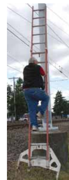
Leveling device clamps onto ladder’s bottom 2 rungs. Bottom of ladder sets in a cradle off the ground and pivots on an adjustable arch.
