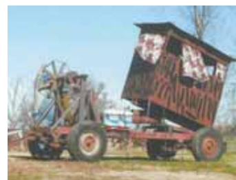
Trailer-mounted deer hunting stand folds down for transport. Holland lowers the deer stand by turning a big wheel that’s welded to a pipe equipped with a cable spool.
