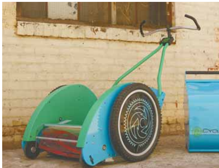
High-speed reel mower has large wheels that drive bicycle-style sprockets.
