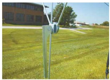
Height of fence line can be quickly adjusted by raising and lowering posts using handtightened clamps. By Loretta Sorensen
