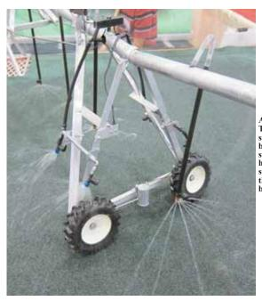
Auto Dry Track System stops ruts before they start by using half nozzles to spray water to the sides and back of tires.
