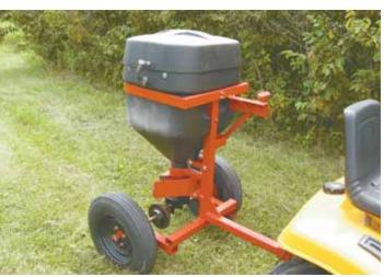
LeRoy Momper built this 2-wheeled, garden-sized fertilizer spreader using the plastic hopper off a pickup-mounted salt spreader.
