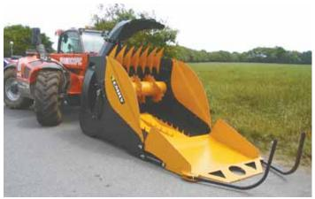
Emily Bale Shredder turns big round bales or big square bales into bedding. Machine can be mounted on telehandlers or big tractor loaders.
