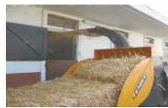
**Unit churns shredded material out through a chute that rotates up to 260 degrees.**
