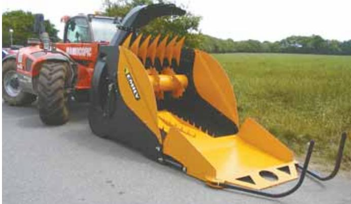
**Emily Bale Shredder turns big round bales or big square bales into bedding. Machine can be mounted on telehandlers or big tractor loaders.**
