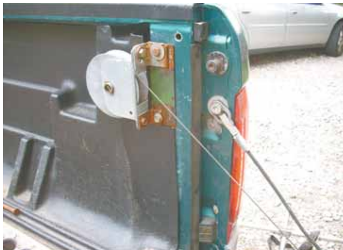
Spring-loaded counterbalancers attach to pickup tailgate, making it easy to close.
