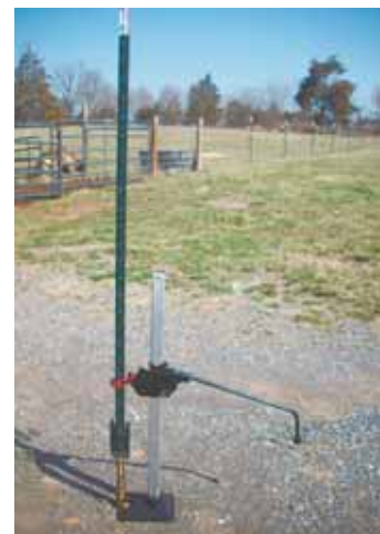
V-shaped slot cut into bumper jack’s base plate allows it to fit around T-post.
