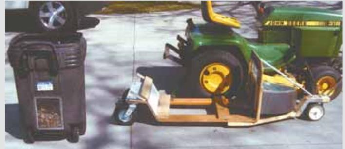
**Cagle's 3-wheeled trailer attaches to discharge side of riding mower, where a 40-gal. plastic garbage can laid on its side (below) collects grass and shredded tree leaves.**
