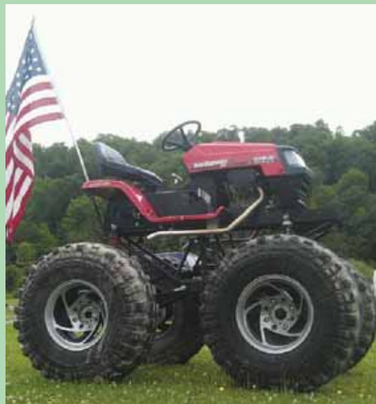
Tony Gernstl's home-built “Monster Mower” rides on 44-in. high lugged wheels off a 4-WD “monster” pickup. The driver sits about 6 ft. off the ground.
