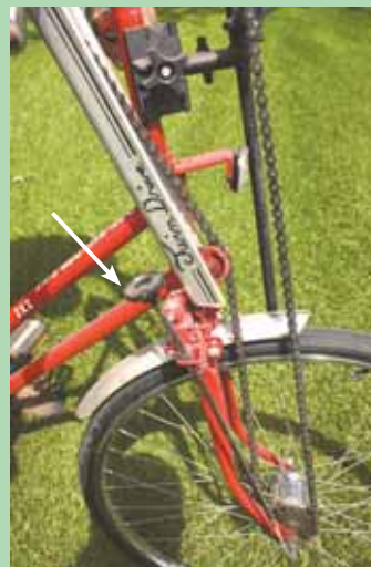
Harold Fratzke invented this “twin drive” bicycle that lets him pedal with either his hands or feet, or use both together. To shift gears the rider pulls on a knob.
