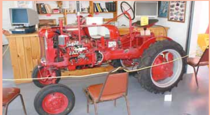
Rare Cub Cutaway was originally used by IH as an educational tool. An electric motor on the tractor ran all the components so you could see how everything worked.
