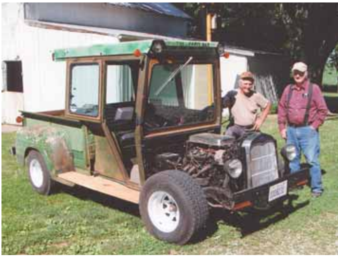
John Eilers mounted an old Deere tractor cab, on the chassis of a Chevy S-10 pickup. Note 1930 Ford Model A pickup radiator on front.
