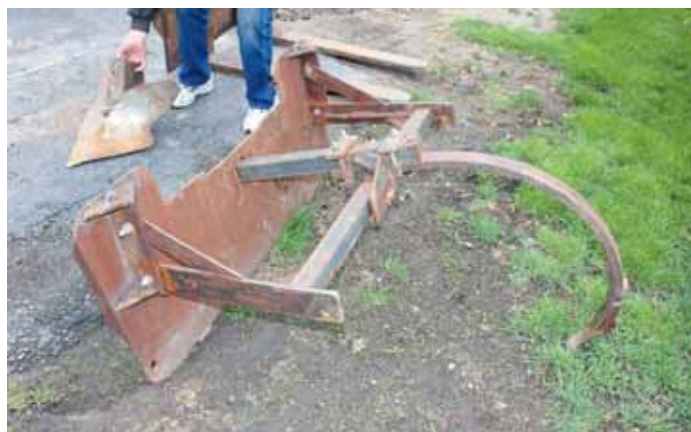
Frank Orr's home-built skid loader-mounted subsoiler breaks up packed soil; then he attaches a bucket to scoop up the dirt.
