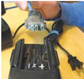
To charge a dead battery, the "dummy battery" is wired with a plug that plugs into the battery to be charged.
