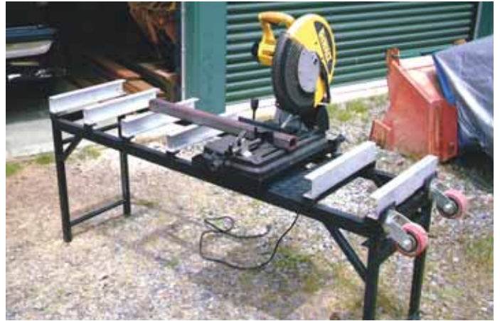
Stew Kunkel made this portable stand that supports his metal chop saw and long pieces of steel to be cut.
