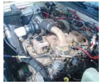
Pickup is powered by a Cummins diesel engine pulled out of an old Frito-Lay delivery truck.
