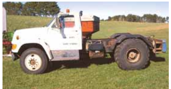
Converted from an old delivery van, "trucktor" is complete with 540 rpm hydraulic pto so the owner can use it to unload chopper boxes at silo.
