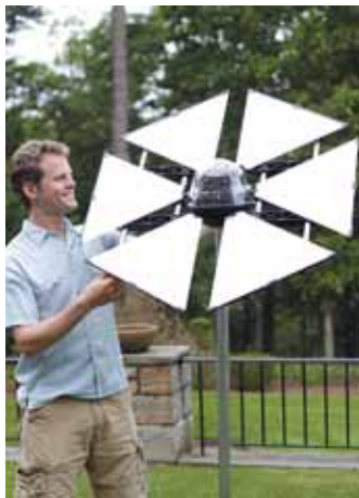
Petal-shaped mirrors mount on a solar-powered tracking device and reflect a focused beam of light anywhere you need it.
