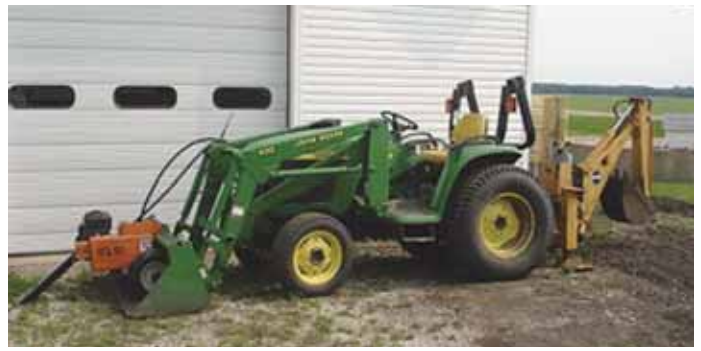
Log splitter is chained to tractor's loader bucket, with quick-connect hydraulic hoses running to tractor's 3-pt.-mounted backhoe.
