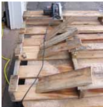
To cut up the pallet Olander uses a chop saw to cut off the cross members, then turns the pallet upside down to repeat the process.
