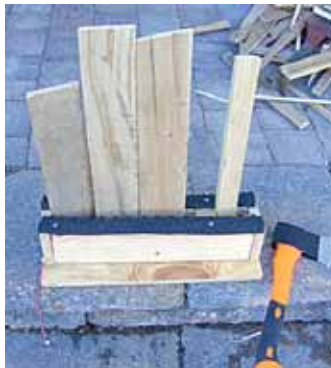
Pallet Kindling Creator holds cut-up pieces of pallet wood, making it easy to split them into kindling-size chunks with an axe.
