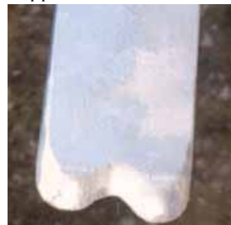
Back side of blade is sharpened.
