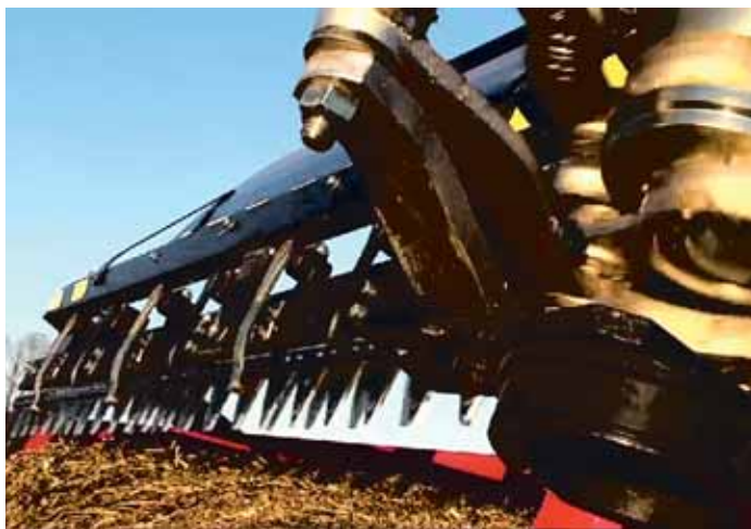
Sam Blank's automated feed slicer cuts hay from big round or square bales with a dual action sickle.
