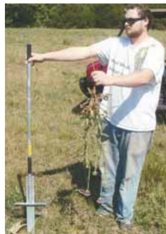
Homemade "thistle kicker" consists of a 9-in. curved metal blade welded to a 1-in. dia. pipe handle.
