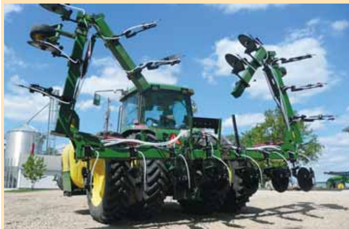
5-ft. hinged extensions added to each end of toolbar allow the rig to cover 16 rows. He uses his Deere 8100 MFWD tractor to pull it.
