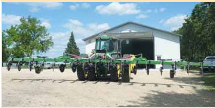
Grant Rollins built this mounted 16-row side dress rig from a used Deere 12-row, 3-pt. mounted cultivator.
