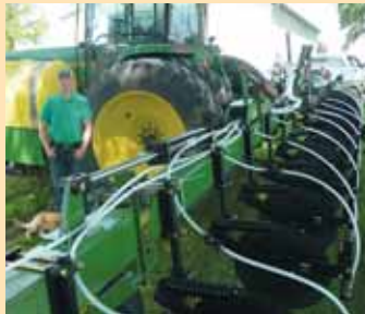
To apply fertilizer, he removed the shanks and gangs from the cultivator toolbar and bolted on Yetter 20-in. ripple coulters.
