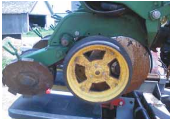
Hoogstraat cut holes into his planter's gauge wheels so they don't plug up with mud. He also converted disc openers into notched closing wheels for better traction in mud.
