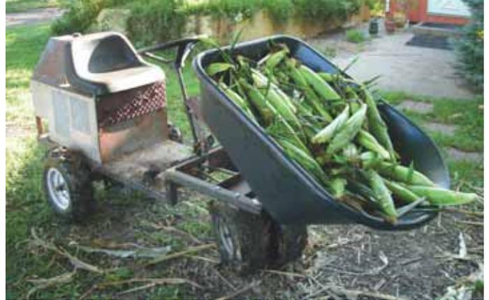
Art Linsenmeyer uses an old riding mower to push a 6 cu. ft. wheelbarrow tub on a tricycle-style frame. Barrel tips toward the front for easy unloading.
