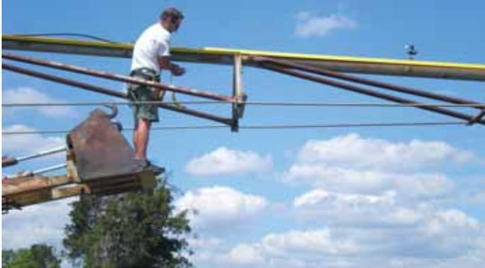
Angle iron, held in place by special clamps, is used to keep thieves from pulling copper wire out of center pivot irrigation systems.
