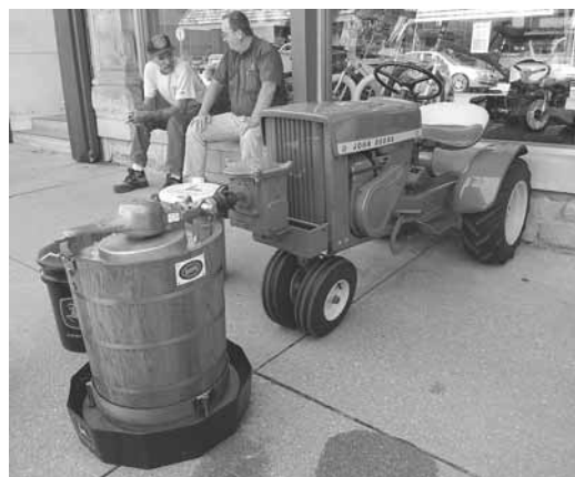
To make ice cream, Michael Densmore mounts a 5-gal. freezer on front of his 1966 Deere 110 garden tractor. Freezer is direct-driven off the tractor engine.
