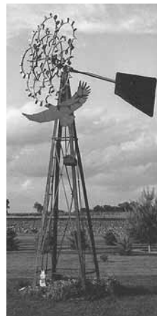
The 30-ft. high windmill's "blades" are made from 8 bicycle wheel rims fitted with aluminum pop cans cut off at the top.
