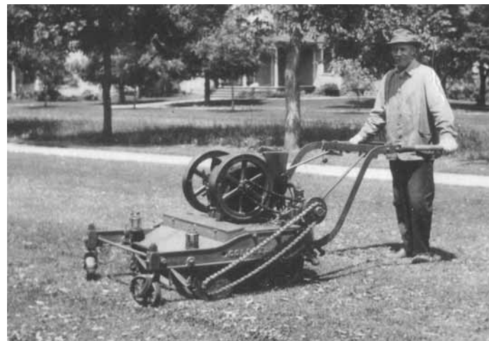
Huge push lawn mower was powered by a Singer gas pump engine. "It was an awfully heavy machine and would have required a lot of effort to operate," says Robert Foster.
