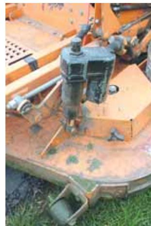
Deck tipper added to zero turn riding mower lets Frank Orr use machine to trim as well as mow. Electric actuator is used to tip front left deck corner of mower.
