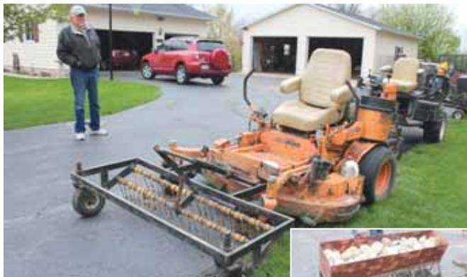
He built a dethatcher to fit on front of the mower (above) and turned a 3-pt. hitch aerator into a pull-type unit.
