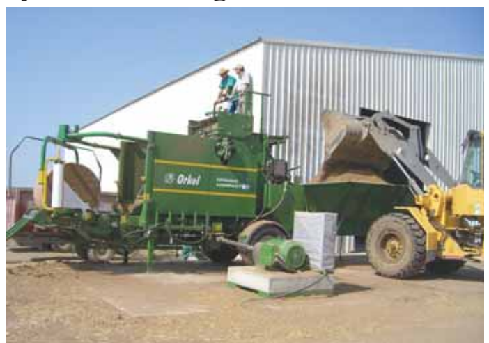
Norwegian-made Orkel baler takes in loader buckets of material at one end and delivers tightly wrapped bales at the other.
