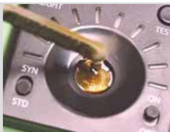
Digital “tester” uses colored LED lights to tell you when oil needs to be changed. You place drops of engine oil from dipstick into sensor’s cup and then press the test button.
