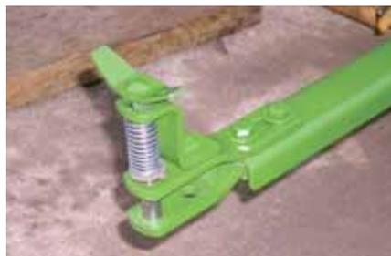
Compression spring holds hitch pin down so it can't shake or rattle.
