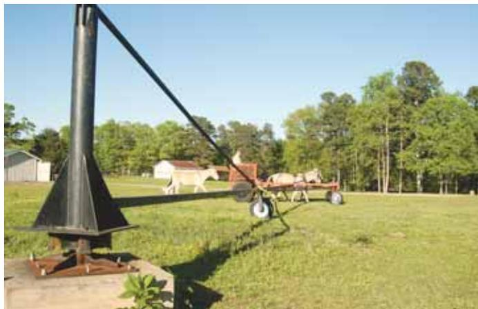
The cart is tethered by a 60-ft. long pole anchored to a truck axle buried in concrete with the wheel hub sticking out.
