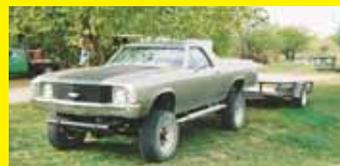
Chevy El Camino body on it. I painted the body silver, with a flat black hood and roof. The El Camino body is bolted onto eight, 4-in. sq. brackets that I welded onto the pickup frame. I added rubber cushions to each bracket to make the ride smoother. I replaced the pickup's original tires with 32-in. tall tires to keep the body from twisting on uneven ground.
