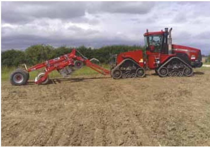
“Sumo” subsoiler is equipped with a central backbone frame that runs front to rear down middle of machine, forming a rigid spine that carries entire stress load.
