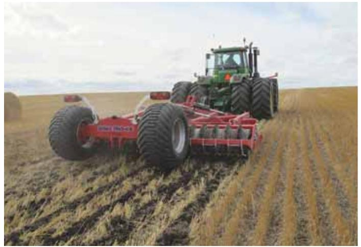
Rig breaks up compaction without digging up the soil too much, leaving the field smooth. It’s available in 7 and 9-shank models.
