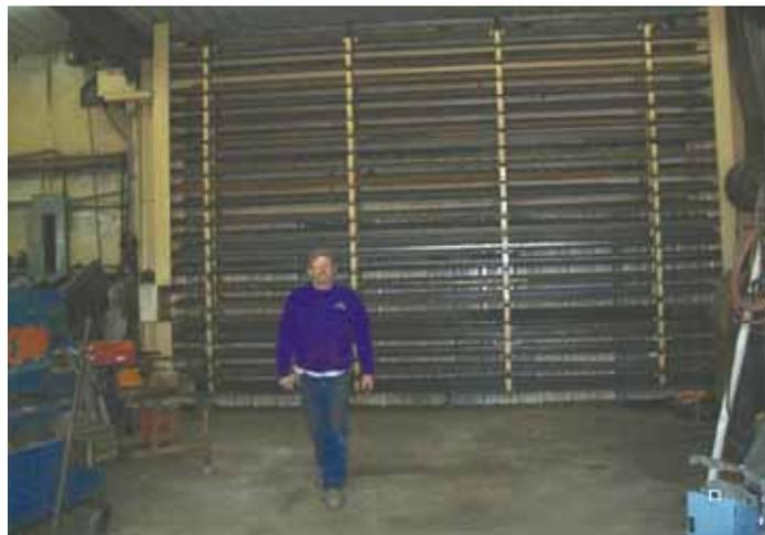
Rotating storage rack is built on the same principle as a continuous loop jewelry display case, maximizing storage space along one wall of Dressman's 75-ft. shop.
