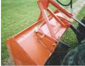
Triangle-shaped steel bracket is welded to back side of loader bucket for 3-pt. hookup. A hydraulic cylinder is used to tilt bucket up or down.
