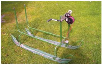
Don Bogardus uses an electric winch to tow this home-built firewood sled up to his house. Hand-cranked winch on sled serves as a backup.
