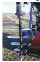
Coneshaped auger makes holes that handle tree balls without additional hand digging.
