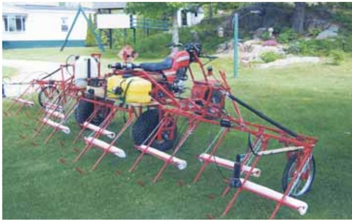
Leon Perry turned a 1985 Honda 3-wheeler into this "high crop" 24-ft. wide wick wiper. Home-built boom bolts onto brackets welded on back of ATV.
