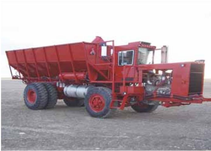
Gerald Bruner and son Brad built this self-propelled grain cart using the frame of a 25-ton Mack "rock truck". They lengthened truck frame 6 ft. on front and 4 ft. on back.
