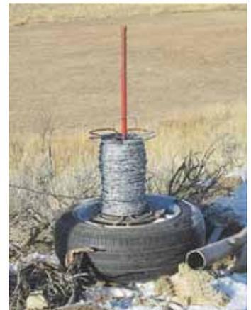
Roll of barbed wire rests on round metal plate on top of wheel rim. Pipe goes down through into the ground a few inches to hold everything in place.
