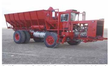
Gerald Bruner and son Brad built this self-propelled grain cart using the frame of a 25-ton Mack "rock truck". They lengthened truck frame 6 ft. on front and 4 ft. on back.
