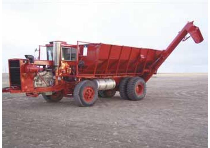
Home-built 900-bu. hopper measures 20 ft. long by 13 ft. wide and was made using sheet steel from old fuel tanks. It's equipped with a 16-in. dia. auger.
