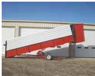
Side view of Olson loading chute (left). A scissors hoist with two 4-in. dia., 30-in. stroke cylinders raises chute up to 11 1/2 ft.
