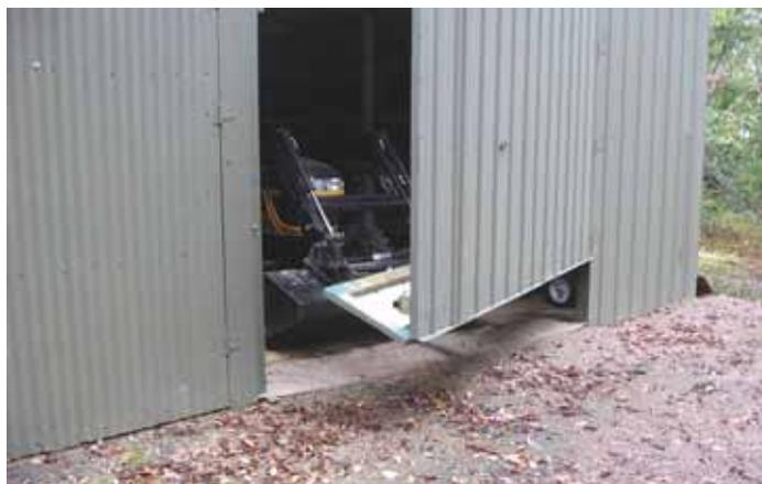
Momper cut through the bottom 2 ft. of his shed door and added hinges. "As I push the door open, the bottom section immediately starts to lift up over snow and ice," he says.
