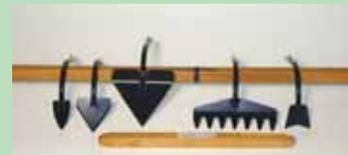
Single, quick-change handle can be fitted with 5 different tools.
