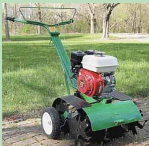
Tiller has 2 shafts. One on front turns forward, and the back one turns backward rapidly to cut weeds into pieces and break up the soil.
