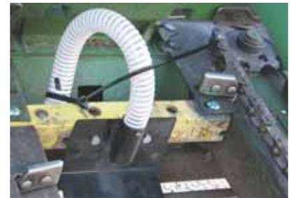
Air hoses emerge over a right angle splash plate that spreads the seed out.
