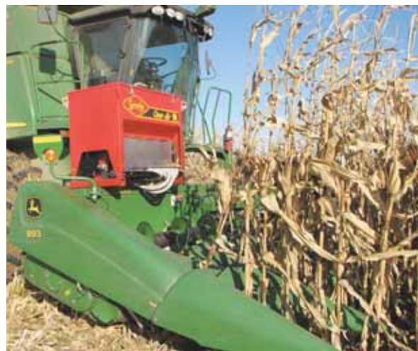
Ray McCormick plants cover crops using a combine header-mounted, Gandy Orbit-Air applicator. "It eliminates the need to make a second trip to plant," he says.
