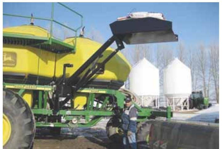
E-Zee Loader uses a hydraulic arm to lift a platform loaded with seed bags from the ground to top of air seeder cart.
