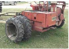
Alan Burda dualed the left wheel on his Gchl 800 2-row silage chopper, adding a 15-in. spacer. "It helps the machine track through muddy corn ground," he says.
