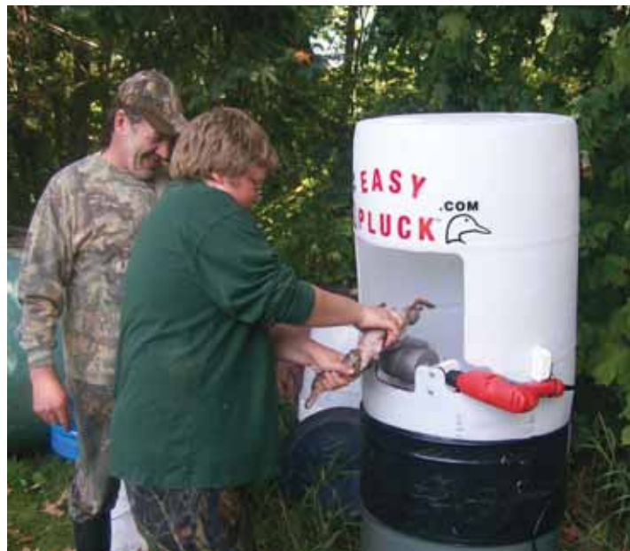
Easy Pluck mounts inside a 55-gal. plastic barrel, which catches all the feathers. Unit is driven by a 3/8-in. power drill.
