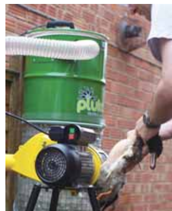
Spinning stainless steel discs pull feathers and the vacuum sucks them away.
