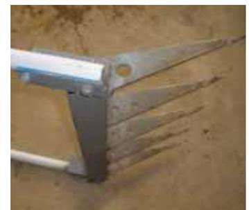
**Teeth look like angled steel "chisels" and easily slice through compacted ground.**
