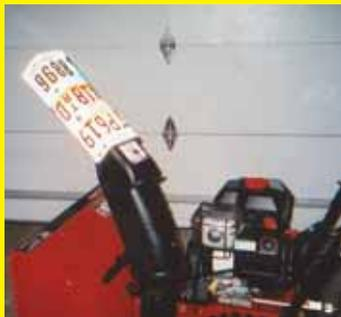
I needed a longer chute for my walk-behind snowblower because wind would often blow snow back in my face. I simply bolted a license plate to the end of the chute and then bolted on two more plates. They're easy to bend by hand and have ready-to-use bolt holes so they easily bolt to each other. **(Steve Cronn, P.O. Box 707, Sundance, Wyo. 82729)**
