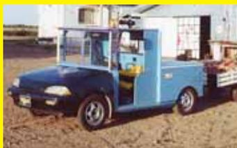
with a turbo, 4-speed transmission, and front-wheel transmission. I had to build a frame and cab out of 1-in. heavy wall tubing and 3-in. angle iron, covered by plywood. The windshield is plexiglass. I lifted the steering wheel and installed tractor seats. The doors are two piece and can be removed in the summer. It has a hitch for pulling a small wagon and
