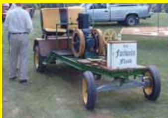
gearbox off an old manure spreader. It rides on a chassis with the transmission, seat and steering gear off a Dodge pickup. Power goes into the side shaft, the rear output shaft connects to the transmission, and the front shaft drives the freezer. The rig can travel at a blistering 6 mph on level ground and 7 mph downhill. It has hydraulic brakes on the rear axle and a lockable cable hand brake.
