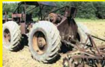
a big steel plate. I welded a 2-pt. hitch on the plate so the skidder can pull disks, harrows and a plow. The winch is used to raise and lower implements.
