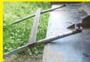
"Here's a photo of a set of forks I built for my Deere loader bucket. I cut holes in a heavy piece of angle iron and weld in two shafts from old hydraulic cylinders, and then weld bolts to the shaft ends. The bolts fit through holes that I cut into the bucket. It's a simple idea but it works great." **(Francis Nemetz, Menominee, Mich.)**
