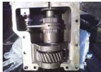
Modified transfer case has a detent spring on the fork shaft, allowing Weaver to slip into 4-WD on-the-go.
