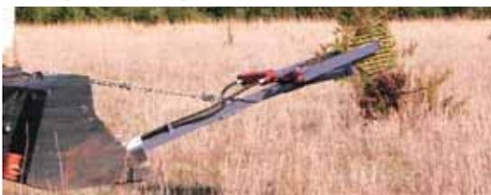
Expanded metal grips can be used to grab brush or pull small trees out of the ground.
