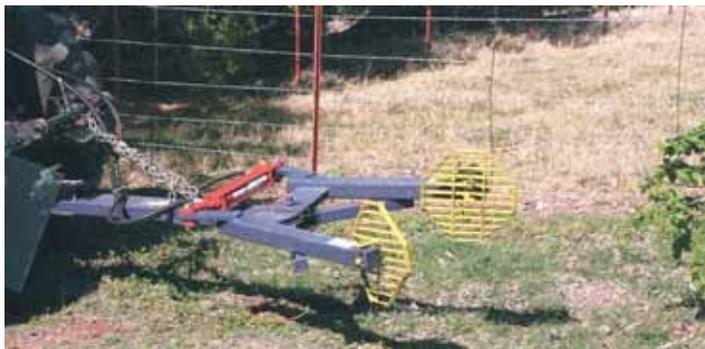
Hydra-Grasp tool has a pair of metal arms equipped with rotating “grips” at the ends. One arm is movable and retracts inward when a hydraulic cylinder is retracted.
